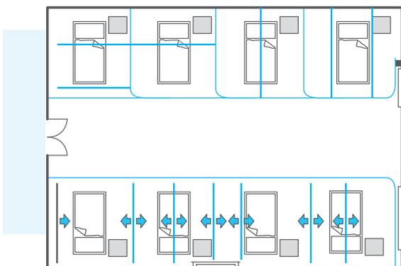
YewdaleMovatrack<sup>®</sup> IV400 lends itself to many configurations within a hospital bed cubicle. The most common configurations of fixed track are shown here, but the specifier should take account of medical factors such as levels of usage, and the possible need of secondary IV provision at the foot of the bed.
